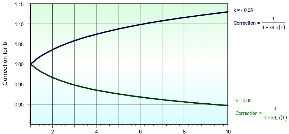
At the start with  $t=1$  is the correction=1. The gradient is here the original one. The interpretation with regard to  $b$  refers to the beginning, while ascertained  $b$  is to be interpreted for 3-parametrig Weibull function approximately on the right outlet of the curve. The Weibull function with correction factor depends on time,  $b$  becomes therefore to:
