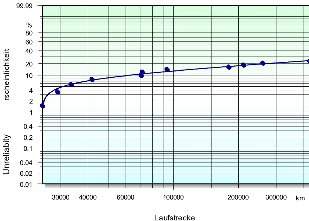
As expected for wearing components, this resulted in a failure-free period  $t_0$ . The shape parameter  $b < 1$ , however, signifies early failures. The apparent contradiction is attributed to the fact that the critical pumps (only 11 out of 47) are subject to a tolerance
