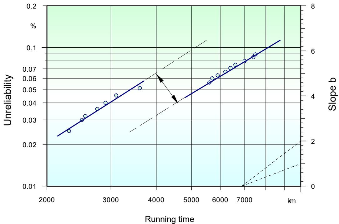
The test used to date would possibly not detect a mixed distribution although the overall slope over all points is not as steep as the individual sections. The concrete example of the above distribution of a starter, however, had definitively different failure causes. In this case, it is advisable to additionally check the respective characteristic life  $T$  in terms of the confidence bound of the overall straight line. This can be achieved by the following approximation formula:
