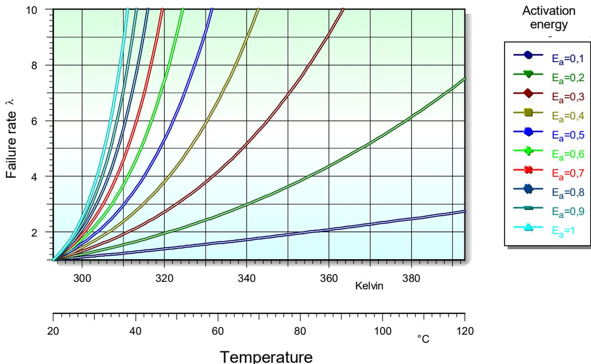
The failure rates increase at higher temperatures ( $T_1 > T_o$ ) and a so-called acceleration factor can be defined:
