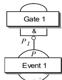
The advantage of the FTA is the hierarchical tree structure. In the upper area you can find the basic connections in the coarser area, in the lower area you can find the details. The FTA thus also provides good documentation of the relationships, even if the probabilities are not specified (qualitative fault tree).
