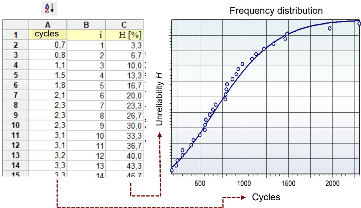
By multiple logarithmic axes you get a straight line. These axes scaling is not possible in MS-Excel. This representation is also called the Weibull net. The frequencies are calculated here using a correction formula, since one assumes a sample in which one does not reach the 100% of the population at  $i = n$ . Here the frequency is therefore  $H = (i - 0,3) / (n + 0,4)$
