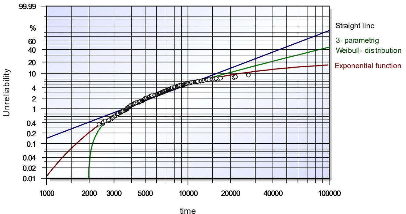
The classical straight line shows the worst approximation of the failure points, in particular up to 10,000 km. The 3-parametric Weibull distribution with  $\tau$  is better quite clearly, however, shows in the outlet of the last failure points still too big divergences. A statement about the failure likelihood, e.g., with 100,000 km would deliver too high values. In this case approx. 45% of failures should be expected. However, these have not appeared later.
