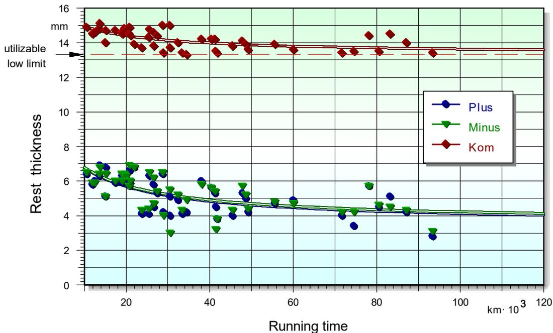
Despite the large scatter or dispersion range, a non-linear relationship can be clearly seen. This means the wear is digressive over distance. This is attributed to the fact that the spring force and therefore the contact force of the positive and negative carbon brush on the commutator decreases with wear. Using a suitable functional approach, attempts were now made to conclude the projected service life. The function
