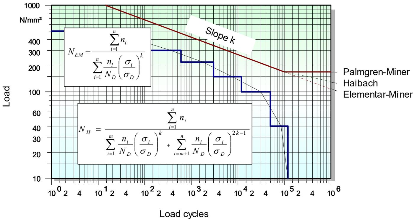
The number of stress cycles that can be borne is calculated in accordance with the elementary Miner rule (EM -> Extension of the slope  $k$ ):
