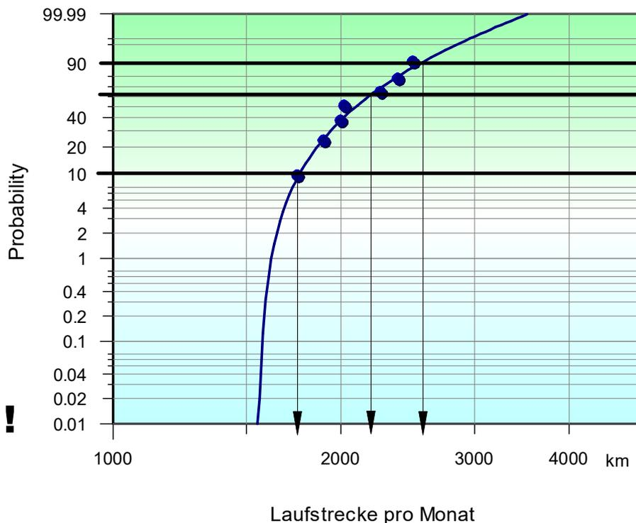
The point of intersection of the best-fitting line obtained from these data at 10%, 63.2% and 90% frequency (probability) provides the required kilometre values at these points. Perpendiculars are drawn at the corresponding frequencies for this purpose (see example). The determined values can now be adopted directly in the actual Weibull evaluation.
