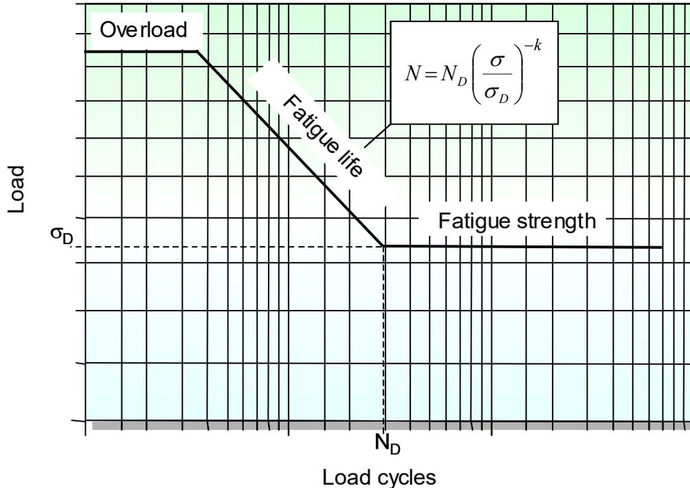
The short-term strength range covers approx.  $10^4$  alternating load cycles. This figure exceeds a load limit at which damage can occur. In the finite life fatigue strength range a diminishing number of stress cycles occurs until fracture) as the load (component stress) increases. This range is a straight line on the double logarithmic scale. The following Palmgren-Miner relationship applies:
