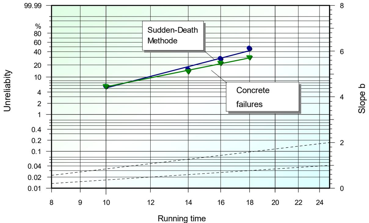
The sudden death method results in a steeper slope than the observation method which takes into consideration only the pure failures (with  $n=12$ ). If, in practical applications, all test specimens were subjected to a test individually and the failures correspondingly plotted, the result would basically that of the sudden death method. The advantage is the considerably shortened test phase.
