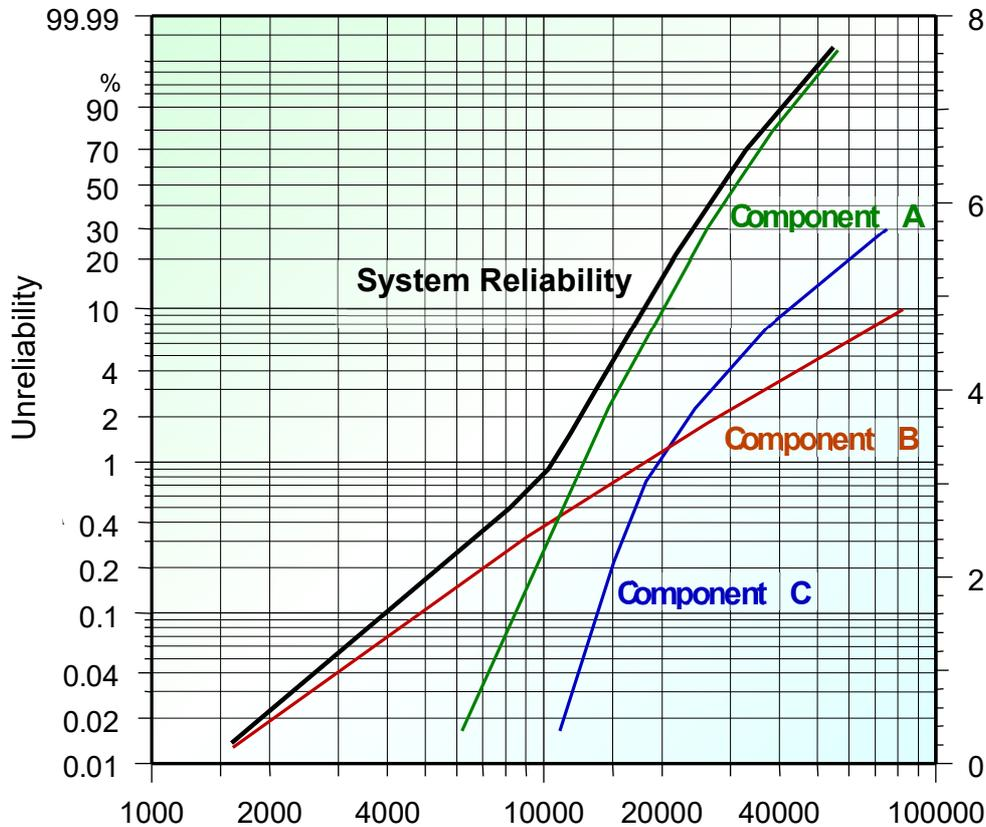
In the illustrated example, component C has a failure-free time. The component B dominates at the beginning, however, component A is decisive in the latter stages. Component B is to be improved accordingly for the purpose of improving the initial situation (warranty period). Component A is decisive for the further reliability over 10000 km.
