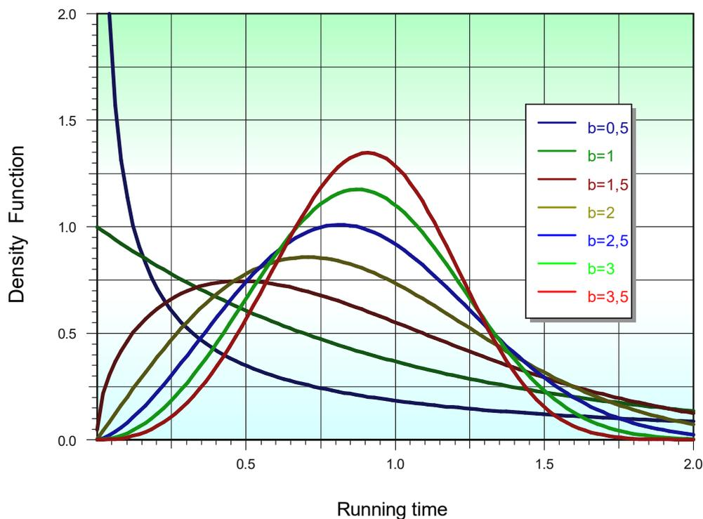
Great importance is attached to the cumulative frequency or the integral of the density function which expresses the so-called failure probability. With this function it is possible to determine how many parts have failed or will fail up to a defined running time.
