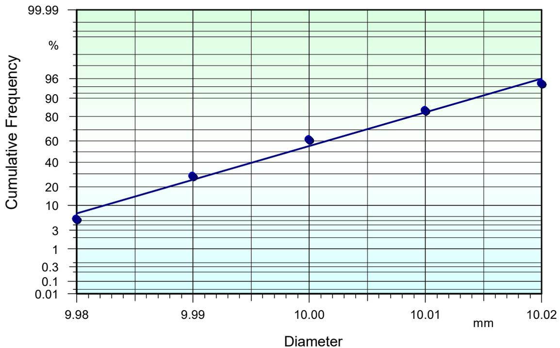
Compared to the frequency distribution, this representation offers the advantage that it is easy to read off the percentage of the measured values within each interval (estimation of percentage of failures outside the tolerance. In addition, it is very easily possible to show how well the values are normally distributed, i.e. when they are as close as possible or preferably on the cumulative curve.
