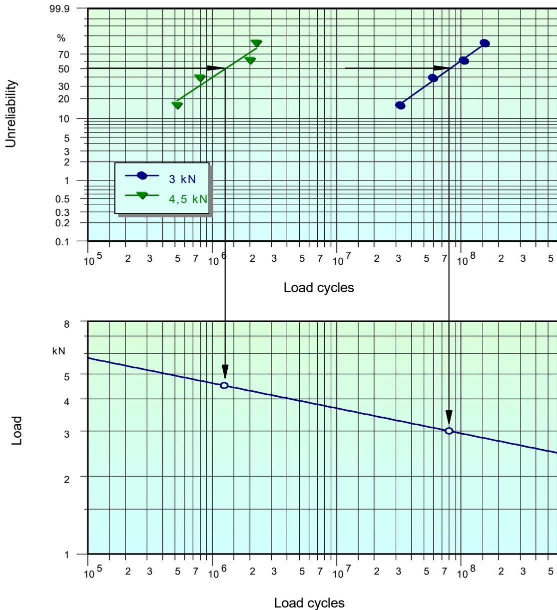
At a certain failure frequency, e.g. 50%, the point in the Weibull diagram is projected downward to the stress-cycle (Woehler) diagram for each load case. The Woehler line can be drawn by connecting these points. In the same way, a probability range can be created in the stress-cycle (Woehler) diagram for a certain range, e.g. 5% and 95% failure probability.
