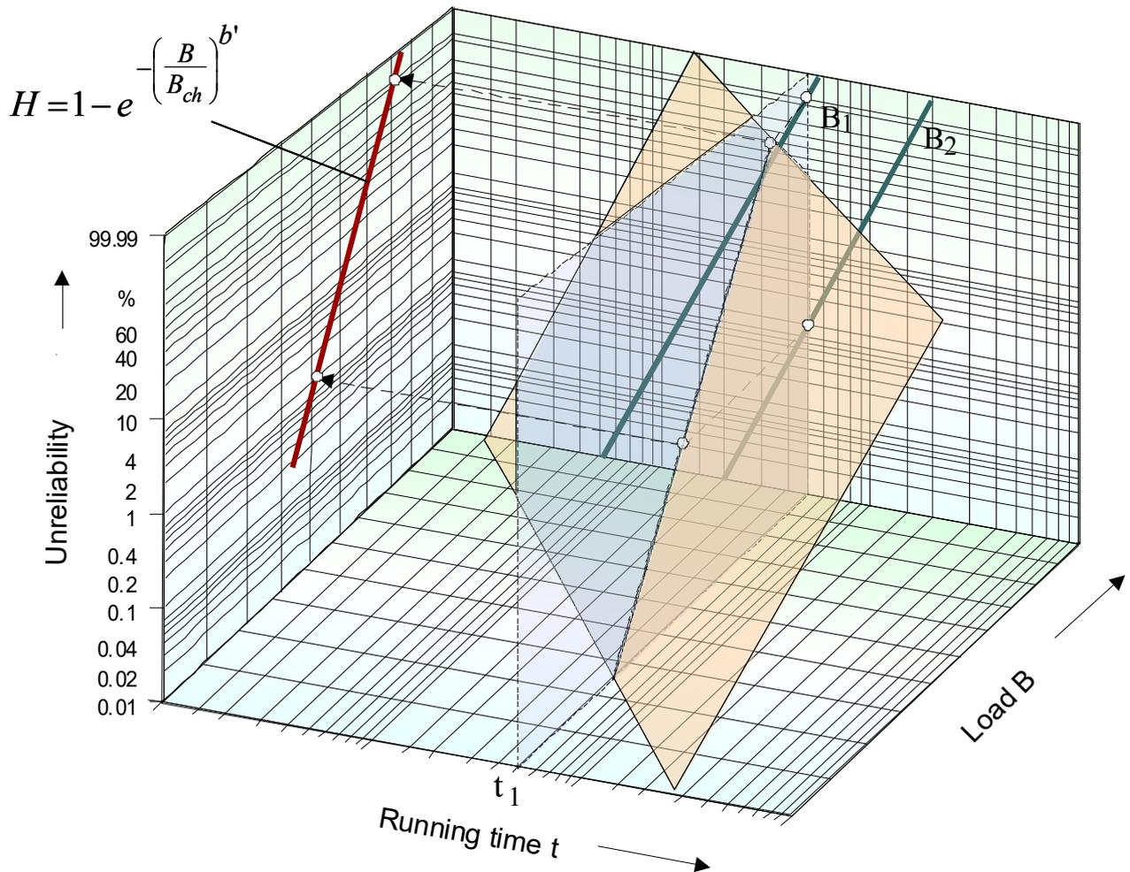
The grey zone represents the relationship between load and failure frequency while the lower level is the stress-cycle (Woehler) diagram. A defined running time  $t_1$  (cutting plane) applies for transfer to the left-hand diagram, resulting in the red curve for which following relationship applies.
