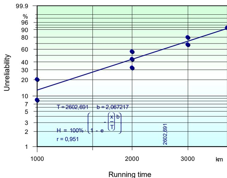
When represented in the Weibull plot as a best-fitting straight line, there are differences in the Weibull parameters attributed to the point distribution in the linearised scale. Although the classification is therefore not incorrect, it is recommended as from a quantity of more than 50 data items.
