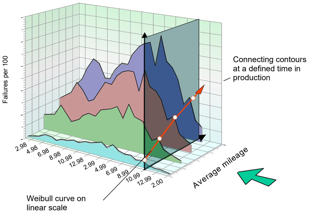
Corresponding to the number of contours, points (red) are obtained for a certain production month. These points can be used to determine the Weibull parameters in pairs (two points are required for the two-parameter form). By rearranging the Weibull functions for  $T$
