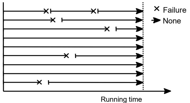
The quantity  $n$  required for the frequencies corresponds to the number of units including replacements. The total quantity originally produced therefore increases by the number of replacement parts.
