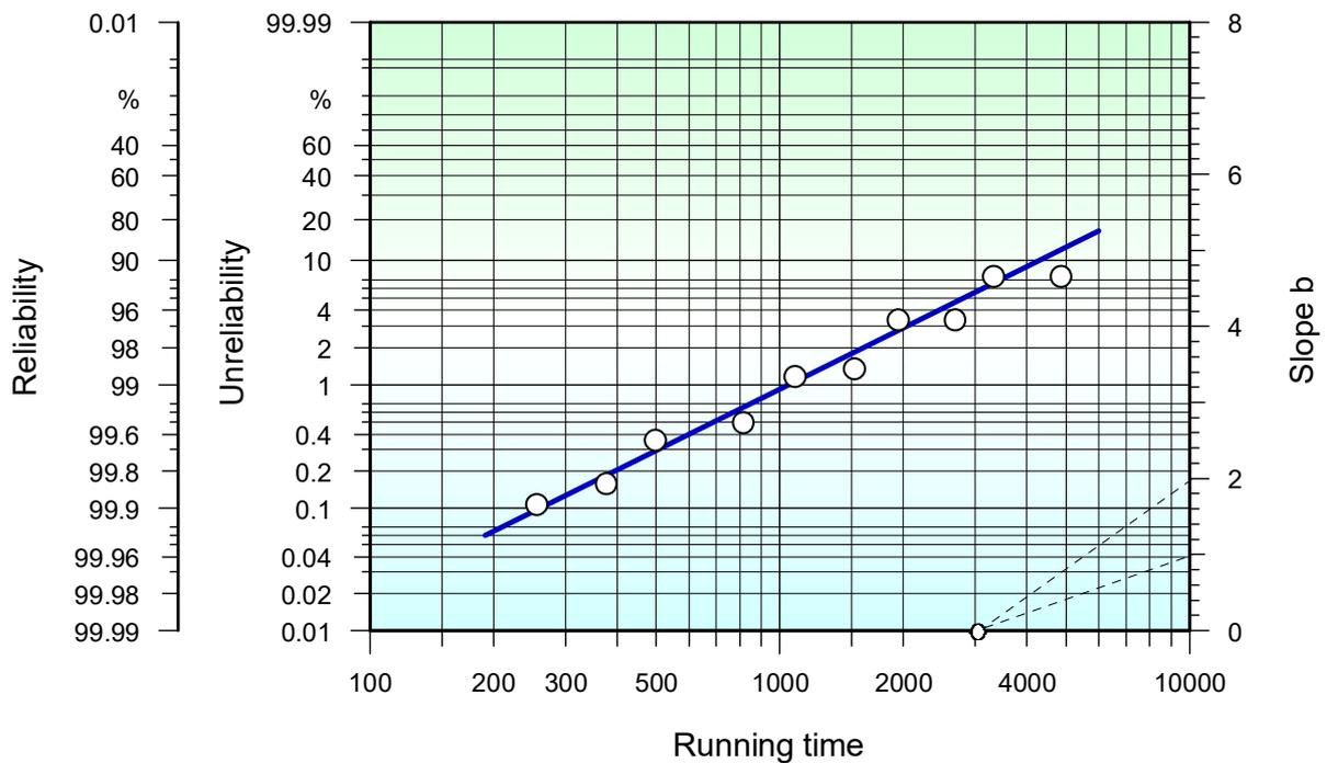
If failure frequencies are low, the specification ppm (parts per million) is also appropriate instead of the percentage. In this case 1% = 10000 ppm.
