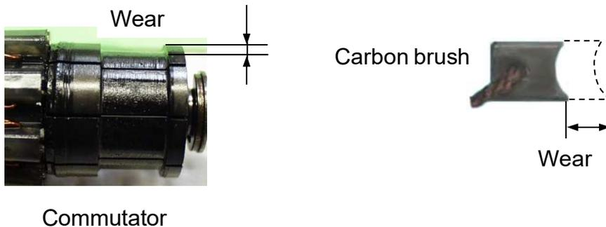
The effective range of the commutator extended up to a minimum diameter of 13.4 mm. The positive and negative carbon brushes were worn when a residual thickness of 0 was reached. Evaluation of the measurements resulted in the following representation as a function of distance (mileage):
