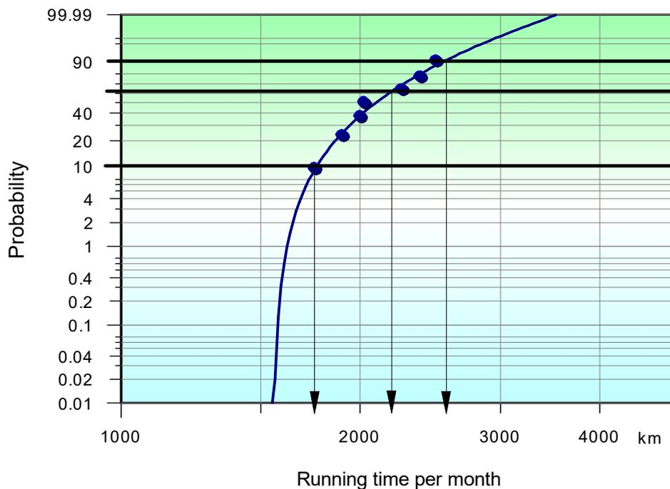
From this representation it is possible to determine how many vehicles have not yet reached a specific mileage. From a mathematical point of view, the inverse Weibull function is necessary at this point (see annex). It is therefore possible to calculate the number of candidates from the production quantity. Let us assume the following concrete failures of a certain component are analysed, sorted in ascending order of distance covered (mileage):
