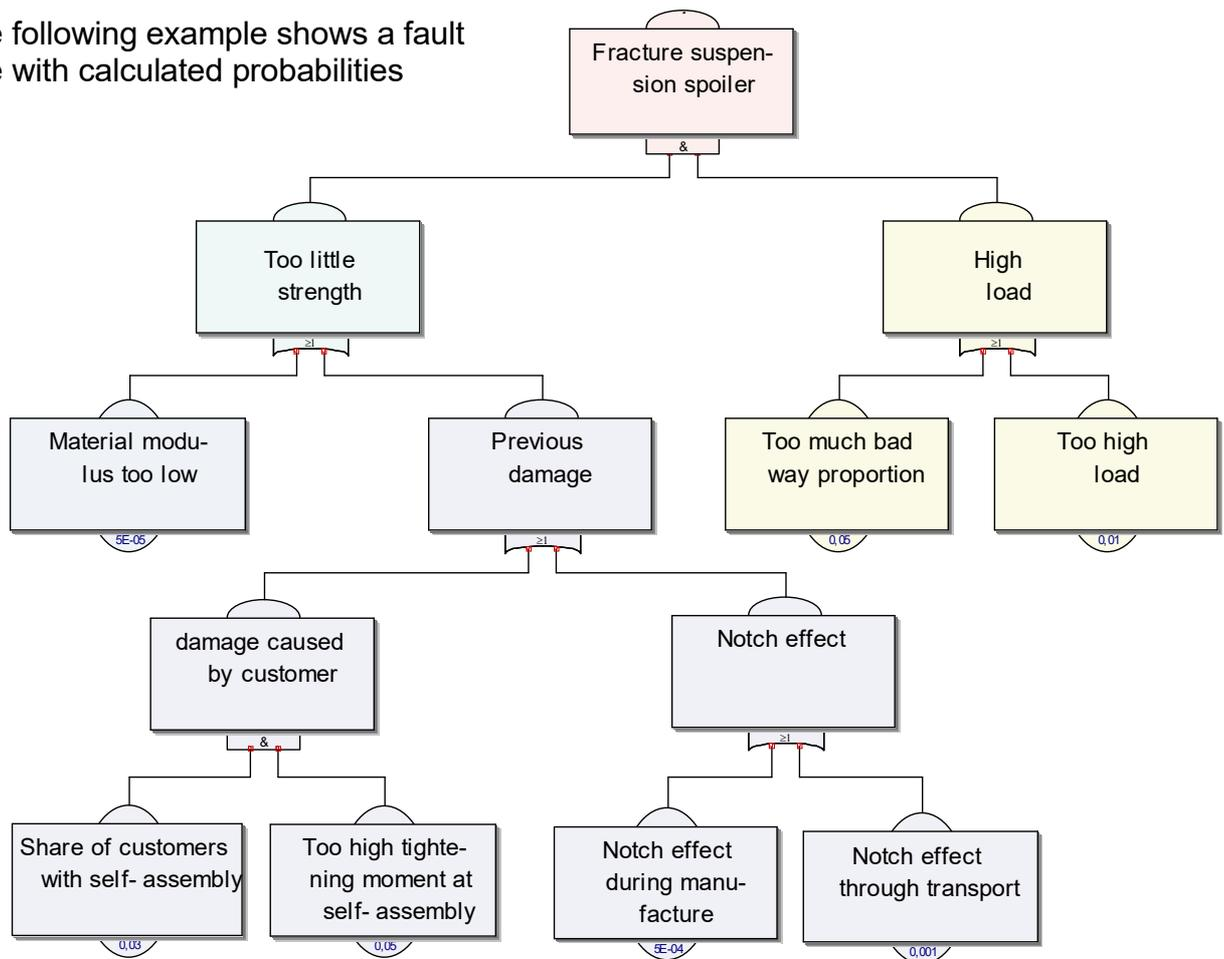
In this example, the system is initially divided into its properties (strength) and what it experiences (load). This is followed by the relevant connections and, at the end, the actual causes (basic events).
