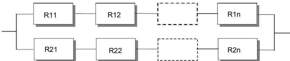
A system fails when at least one component has failed within both series-connected power trains.
